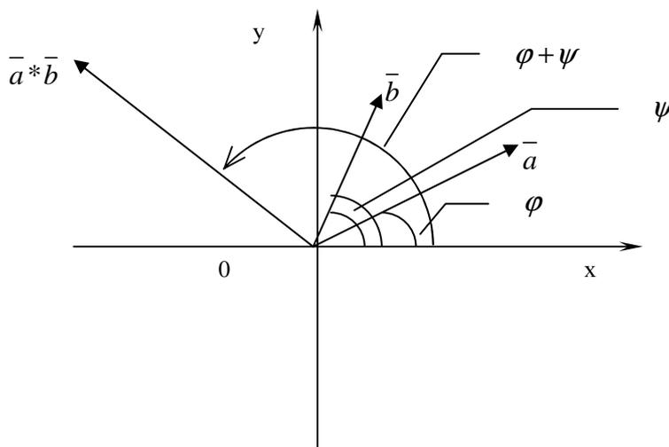
$$\begin{aligned} \frac{a}{b} &= \frac{r}{R} \left( \frac{\cos \varphi + i \sin \varphi}{\cos \psi + i \sin \psi} \right) = \frac{r}{R} \left( \frac{(\cos \varphi + i \sin \varphi)(\cos \psi - i \sin \psi)}{(\cos \psi + i \sin \psi)(\cos \psi - i \sin \psi)} \right) = \\ &= \frac{r}{R} \frac{\cos \varphi \cos \psi + \sin \varphi \sin \psi + i(\sin \varphi \cos \psi - \cos \varphi \sin \psi)}{\sin^2 \psi + \cos^2 \psi} = \frac{r}{R} (\cos(\varphi - \psi) + i \sin(\varphi - \psi)) \end{aligned}$$
